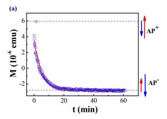
Fig. 2. Magnetic relaxation in Pt(3 nm)/Co(1.05 nm)/Ir(1.5 nm)/Co(0.7 nm)/Pt(3 nm) in the magnetic field – 1350 Oe at T = 100 K. Here  $M(t) = M_{S1} (-x-0.3y+z)$ , where  $M_{s1}$  is the saturating magnetization of the thick layer. The solid line is the exact solution of (1), the blue circles — the results of the observations (for further details see [13])
