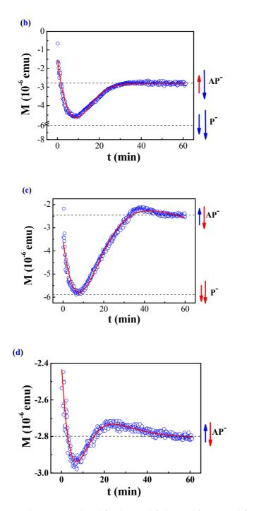
Fig. 3. Magnetic relaxation in Pt(3 nm)/Co(1.05 nm)/Ir(1.5 nm)/Co(0.7 nm)/Pt(3 nm) in the magnetic fields – 1360 Oe (b), – 1354 Oe (c), – 1370 Oe (d) at T = 100 K. The solid lines are exact solutions (16), the blue circles – the results of the observations (see [13])
